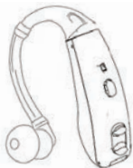
1 Ranger®-6670 hearing aid with pre-cut tube and MS BTE dome attached
